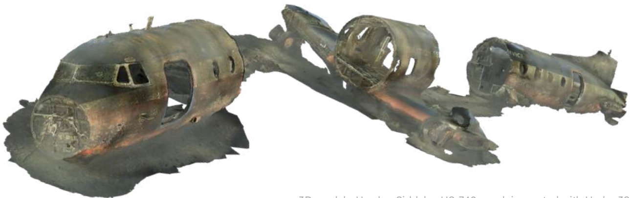
3D model - Hawker Siddeley HS-748 wreck inspected with Hydro 300
