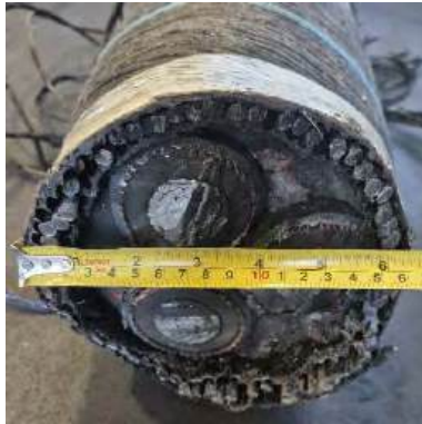
150mm armoured export cable cut by MicroPAQ.
