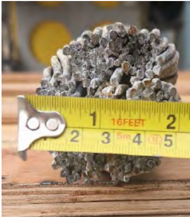
50mm wire rope cut by MicroPAQ.
